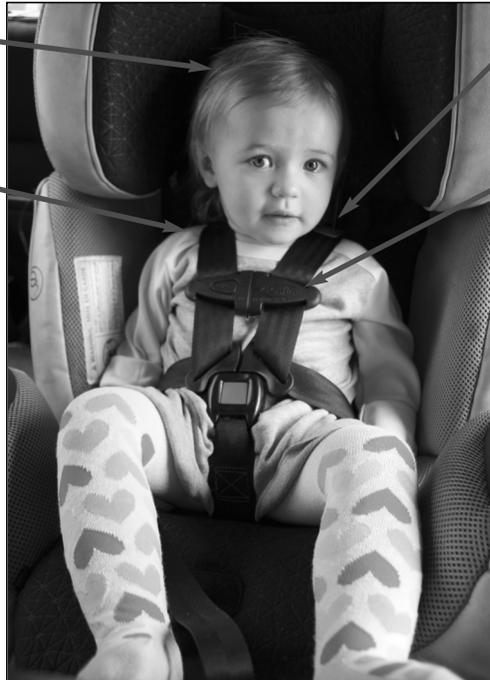
Harness should be at or below shoulder level and threaded correctly.
