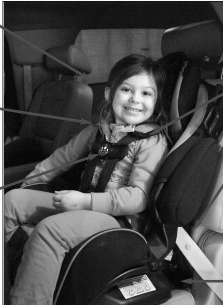
Tether anchor strap used if anchor is provided in the vehicle.
